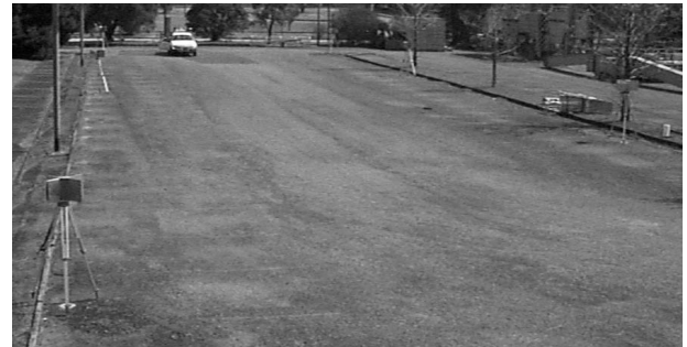
Fig. 3. Test vehicle at the test site. A radar point landmark can be seen in the left foreground
